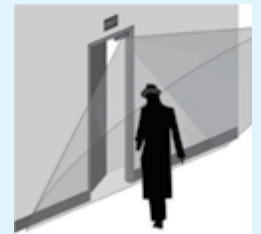
Embedded CCTV captures full facial view of persons exiting door
