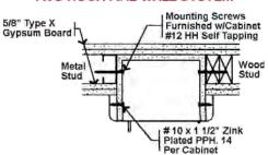
UL Classified 5/8" Type X gypsum board inserted in the cavity between the two layers. Warnock Hersey has approved the Safeguard Cabinets to be mounted in any face of fire rated steel or wood stud for up to 2 hour rated walls without affecting its fire rating. The above meets the requirement test ASTM-E119-98 with test report WHI-495-1534. MOUNTING INSTRUC-TIONS are supplied with each safeguard cabinet.
